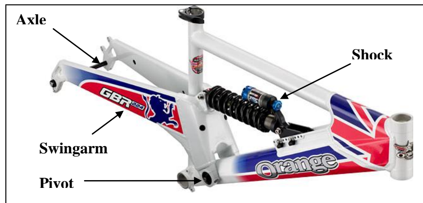
Figure 1 Single Pivot Design (from Orange Bikes (3) )
