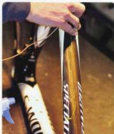
This road frame had obvious top tube damage from a handlebar impact. In this case, Raoul found delamination way back at the seat tube junction—it's unlikely that this would have been detected without ultrasound.
